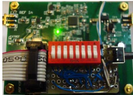
Figure 1. Orion PLL, with coverage from 35 to 4400 MHz
