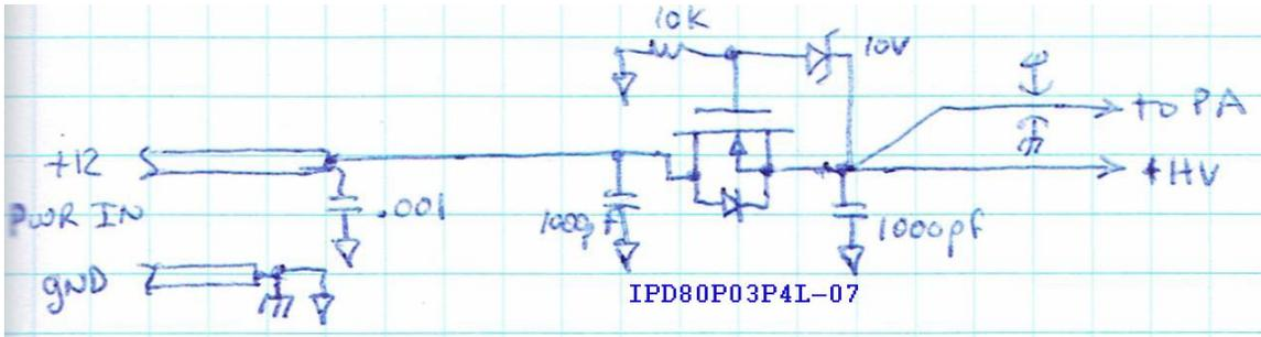
Power input and reverse polarity circuit.
