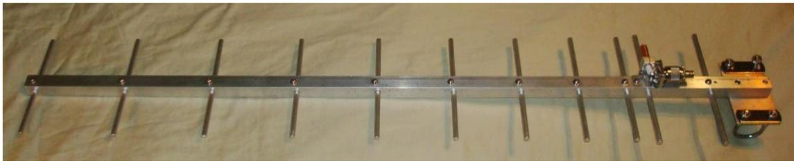
Figure 4. 11 element, home-brew beam for 902 MHz
