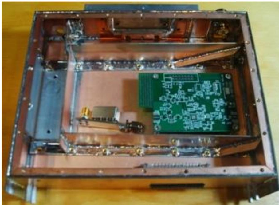
Figure 3. 902 TX chassis mock-up
