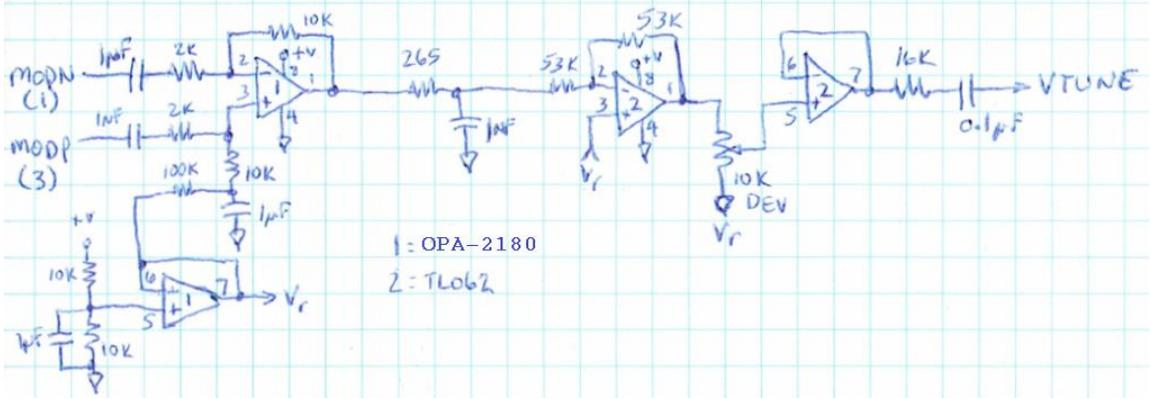
Modulator buffer and conditioning circuit: The 265Ω and 1μF capacitor (a film type) form a 600 Hz LPF to counter-act the HP effect of the PLL loop filter.
