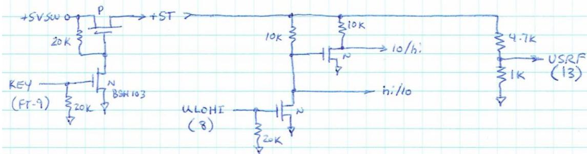
KEY and High/Low power logic: USRF presents a small voltage in TX and 0V in RX so that the IC-901 RF/SMET indication is correct.
