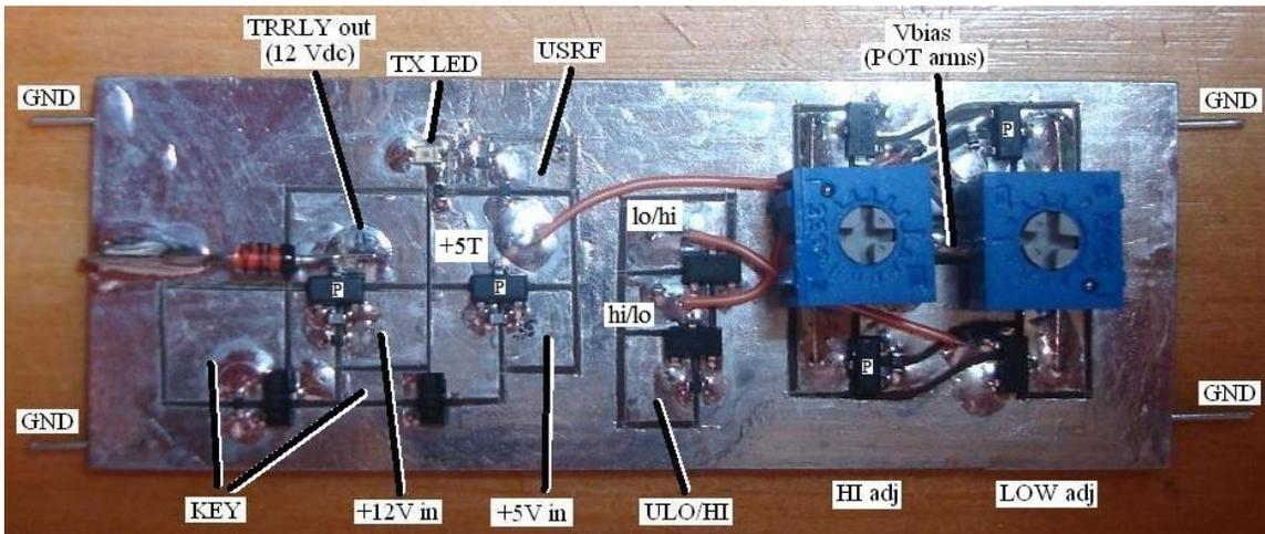
Main logic board: Contains the T/R relay driver, S/RF level, and VBIAS (HIGH and LOW) adjust. The TX LED is for debug use and is not placed for viewing in normal operation.
