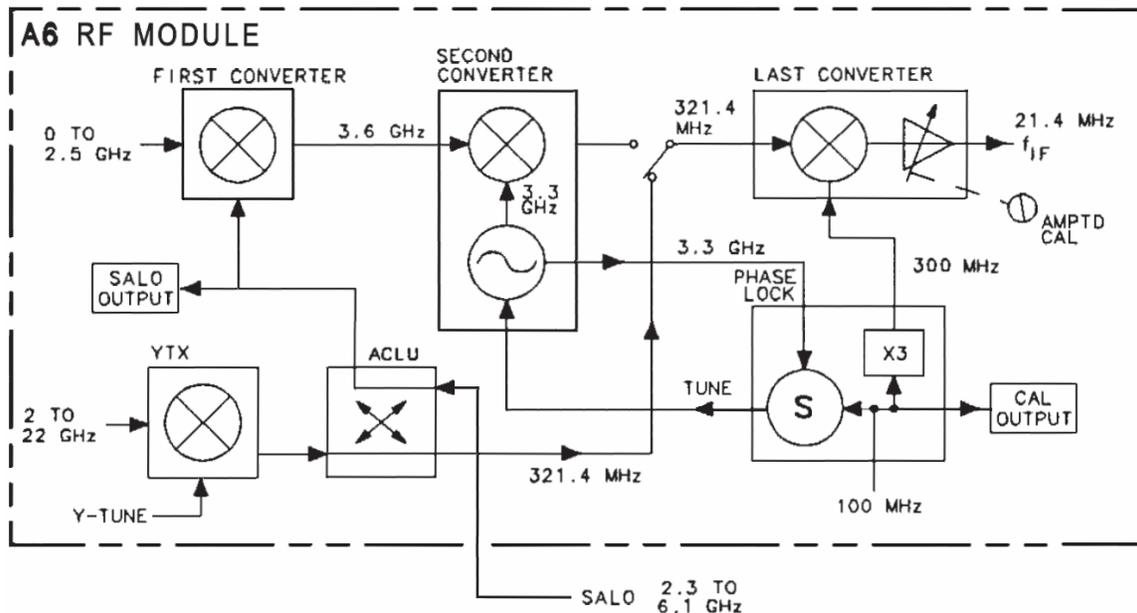
Figure 2. Simplified Block Diagram of the HP-8566B
