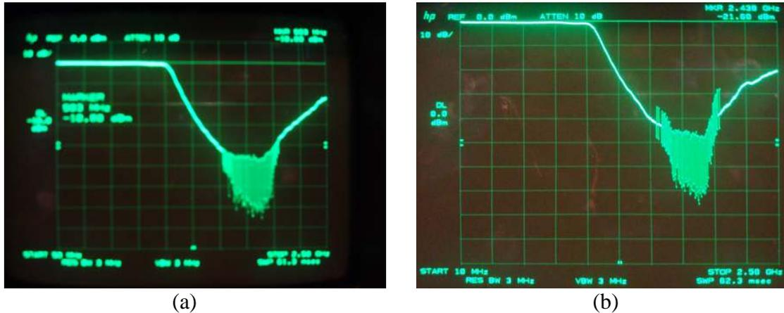
Figure 9. Normalized SNA plot of a MiniCircuits PLP-1000+ LPF with (a) 16dB of attenuation in the DUT chain, and (b) 10 dB of attenuation.
