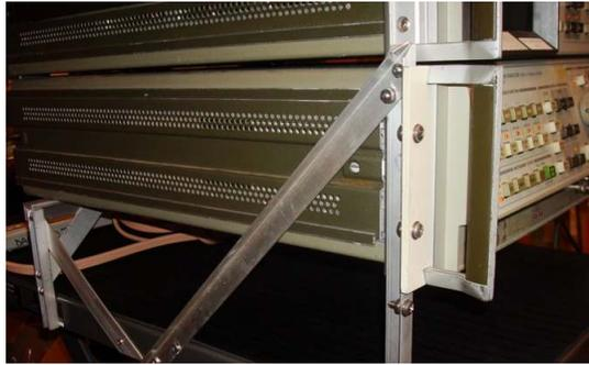
Figure 4. HP 8566B lit-cart rack-mount structure
