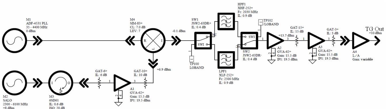
Figure 7. Block Diagram for the T/G signal chain
