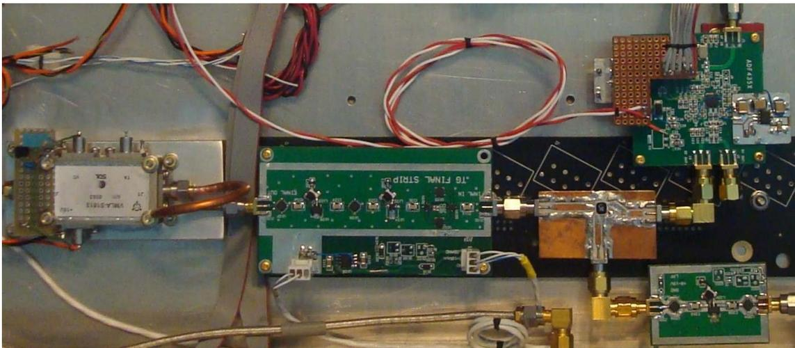
Figure 8. T/G RF subassemblies. From the upper right clockwise: TGLO source, ISO-AMP, MIXER, Final strip, and Levelling Amp.
