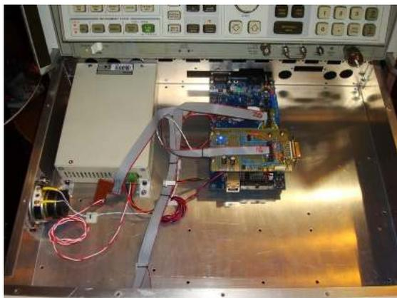
Figure 5. T/G Chassis with power supply and GPIB controller installed
