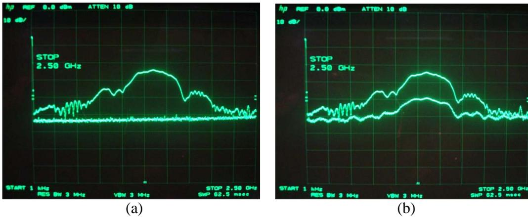
Figure 3. At (a), the S/A response with the T/G mixer active (top) and inactive (bottom). At (b), the S/A response with no attenuation between the isolator and T/G mixer (top) and with 10 dB of attenuation (bottom). All traces are max-hold.
