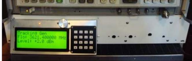
Figure 6. T/G front panel (minus RF connectors). The SALO output can be seen just to the left of the main S/A input
