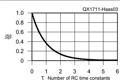
Figure 3 — This voltage versus time-constant plot for a capacitor may be used to graphically determine a value for  $C$ .
