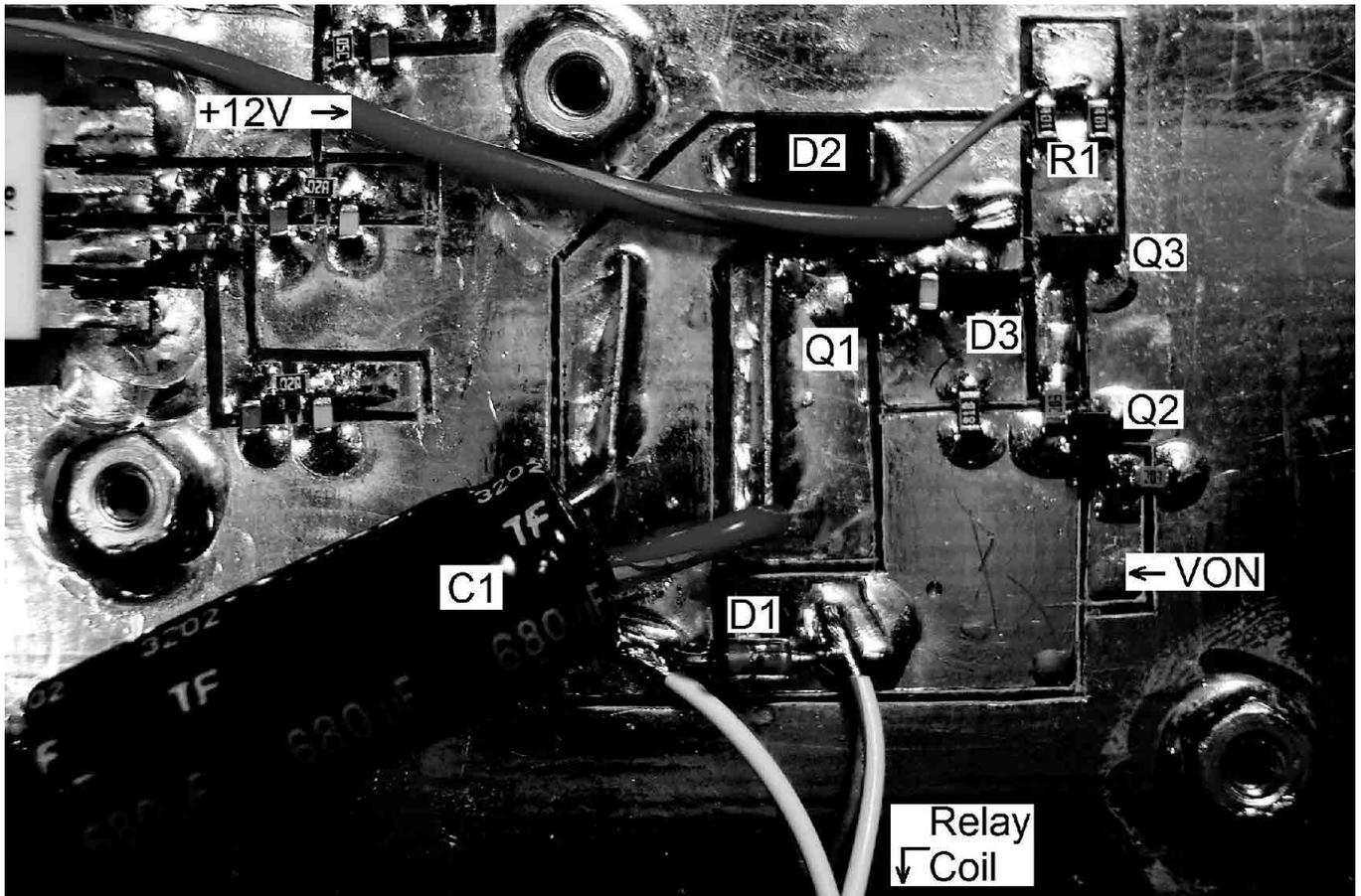
Figure 6 — Photo of an implementation of the circuit of Figure 5. The power-on set circuit was not use in this implementation. The area surrounding the circuit is ground.
