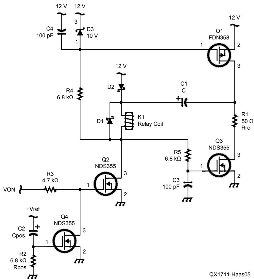
**Figure 5 — Digitally controlled relay drive circuit. The  $+V_{ref}$  is a regulated voltage reference. An unregulated reference may be used, but the highest likely  $V_{rel}$  voltage must be used to calculate the value of  $C_{pos}$ .**
