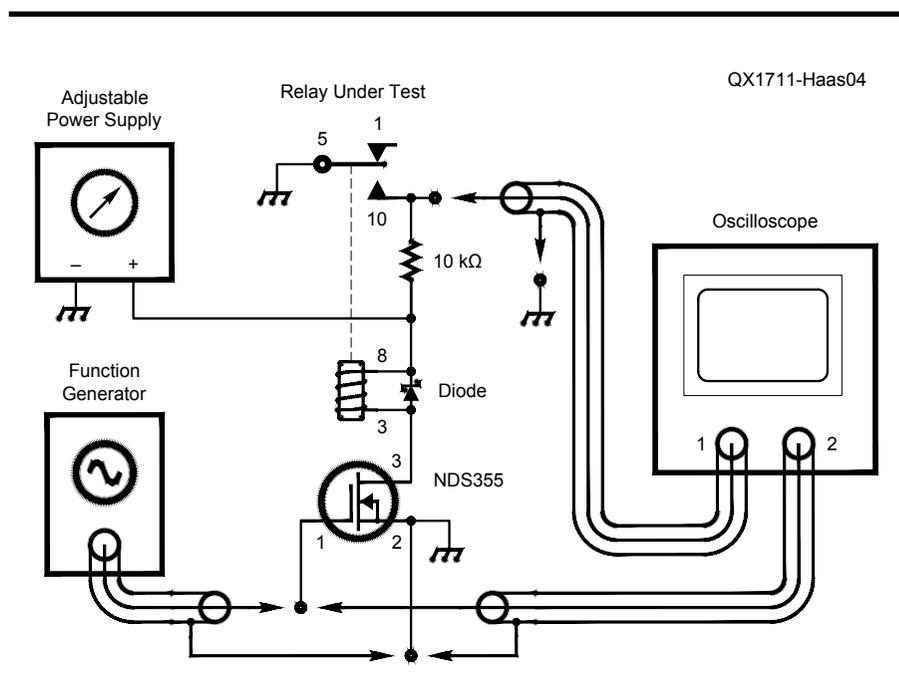
Figure 4 — Test setup for measuring critical relay parameters.
