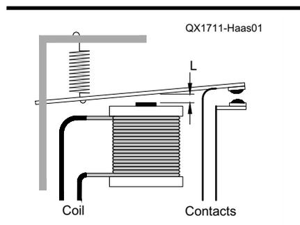
Figure 1 — A simplified relay system.
