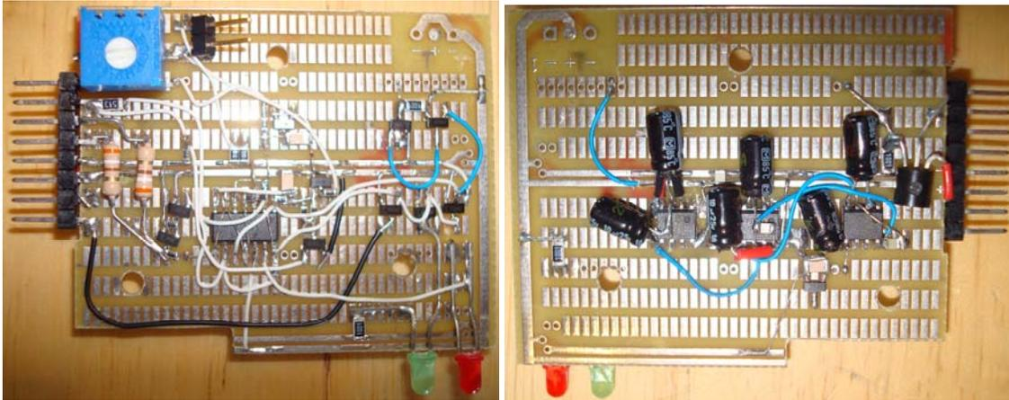
Photo 1 (a & b). Control card. Left (top of card) is the comparator switch circuit. The right image (bottom of card) is the -24V bias supply. The proto-board is a custom design that I produced specifically for SOIC/0603 prototype circuits.
