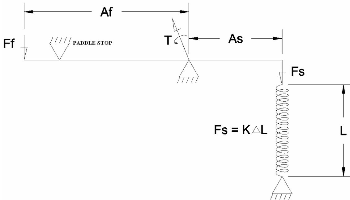
Figure 2. Moment vs. Force free-body diagram (the direction of  $T$  is perpendicular to the plane of the page)
