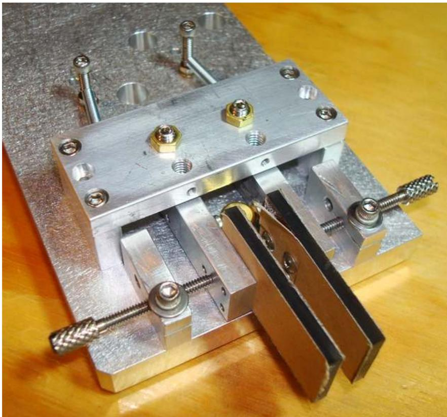
First test-assembly with all of the major pieces in place. The springs attach to 1/2", 2-56 screws that thread into the side of the paddle arm pieces. Yet to do: the finger pads need to be finished, the brass shoulder screw needs to be Ag plated, and the gap-adjust finger screws need to be shortened. Also, an optional shield plate will attach to the top of the axle support piece. This will serve as the "table top" when the keyer assembly is in its installation configuration.
