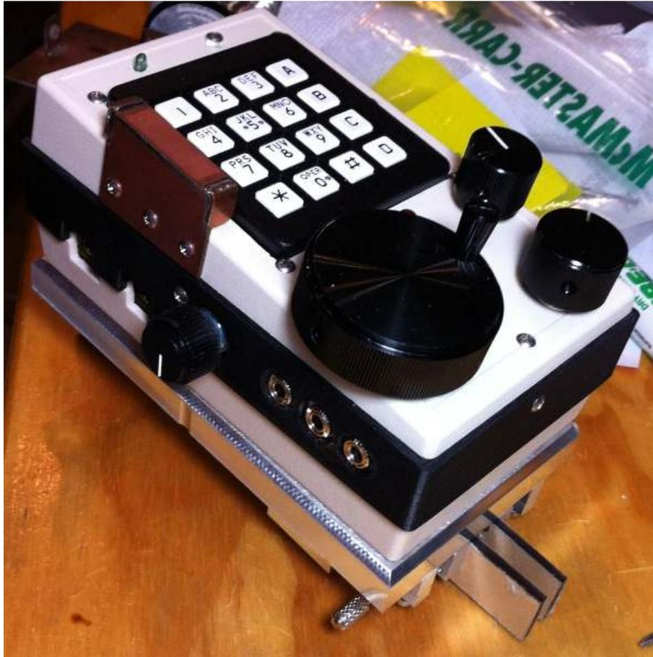
Mockup of the keyer paddles in their installation configuration. The keypad unit above is part of the user interface to the system controller.
