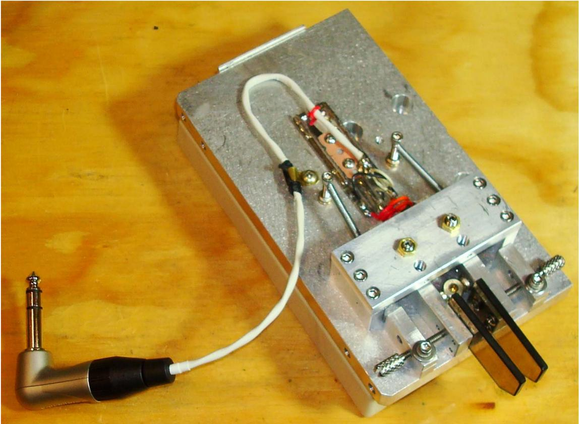
Finished Paddle Assembly (shown up-side-down). The short cable connects to the keypad unit that installs on top of this assembly. A wedge-lock is used to attach the keypad unit to the top of the paddle base-plate (the lower section of the keypad enclosure can be seen attached in this image).
