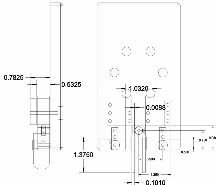
Figure 1. CAD drawing of keyer-paddle assembly
