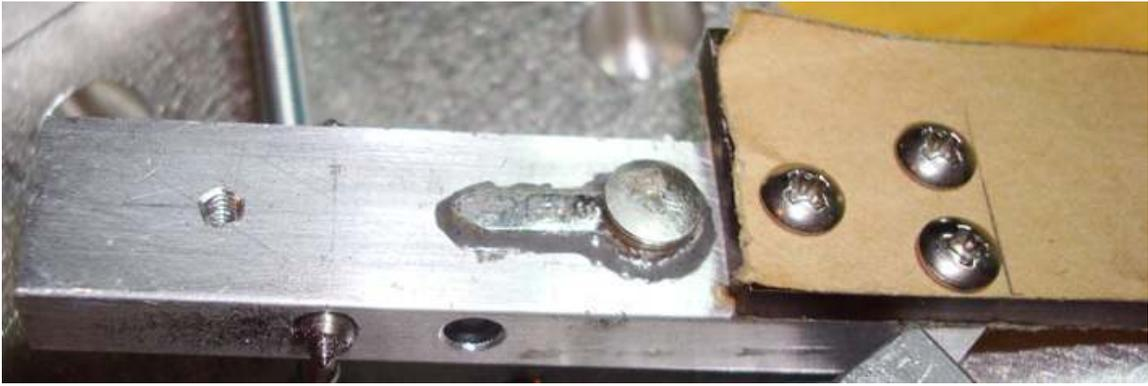
Close-up of one of the paddle assemblies. The contact is soldered to a 0.062" thick piece of FR-4 material cut to match a milled out depression in the arm. A wire will be soldered to the left side of this contact assembly and routed to a terminal on the baseplate.
