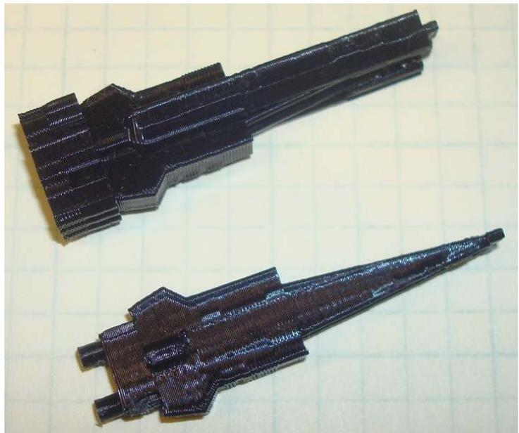
Figure 2. 3D printed “clone” of the ICOM optical connector. At top: the housing with printed support structures. At bottom: the housing after clean-up.
