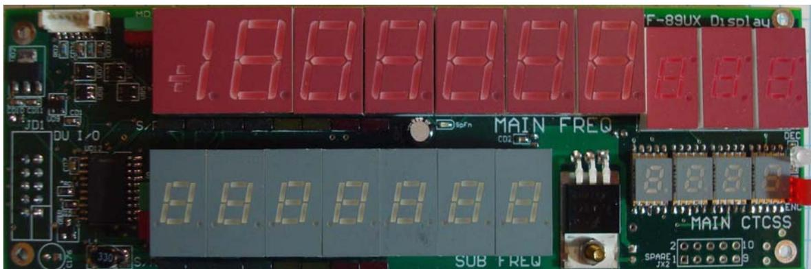
Figure 4. Display module, assembled
