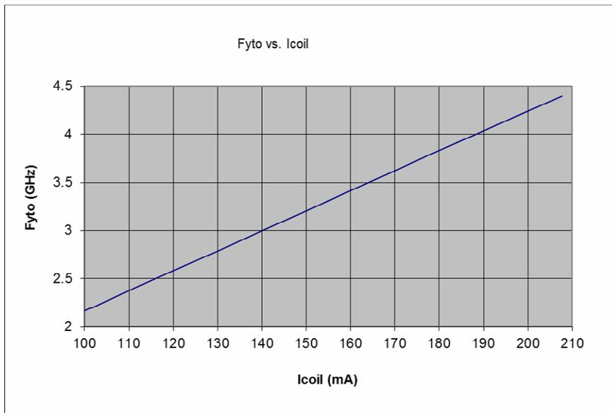
Figure 1. YTO  $F_{out}$  vs.  $I_{coil}$
