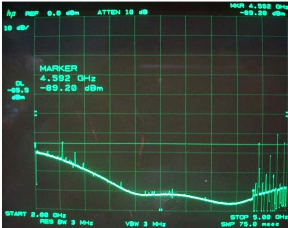
Figure 4. Swept YTO plot of a microwave isolator using the FM and pre-tune coils.
