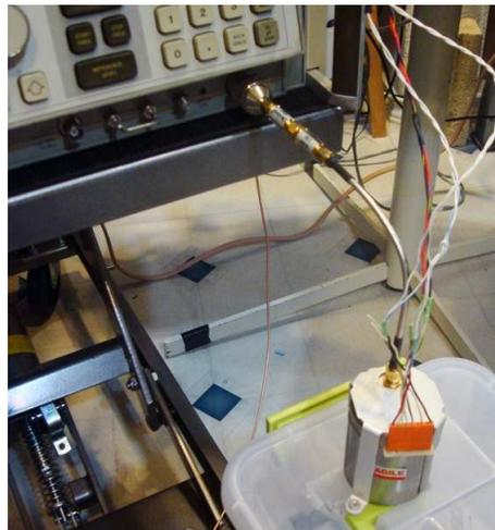
Photo 4. RF Test set-up. Note the 6dB and 10dB attenuator in line with the YTO output.
