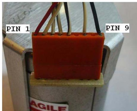
Photo 2. YTO connector close-up view.
