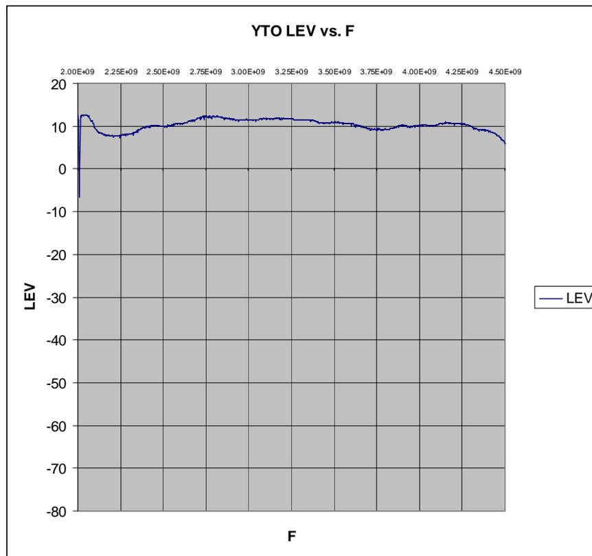
Figure 2. YTO Output (dBm) vs. Frequency (Hz)
