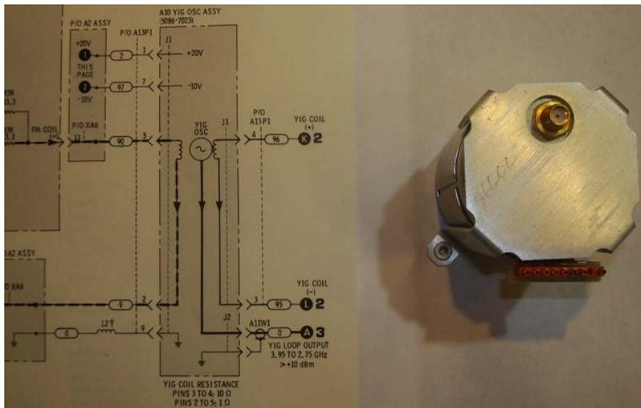
Photo 1. The 5086-7023 YTO and a section of the HP 11661B schematic showing the YTO pinout.
