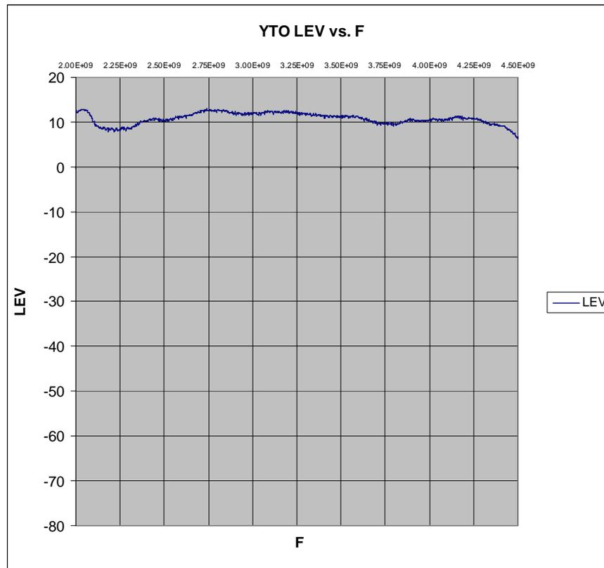
Figure 3. YTO output vs. frequency after 2 hour warm-up.
