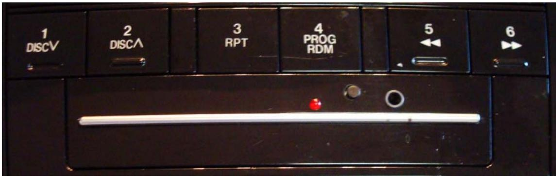
Stereo buttons. Buttons “3”, “4”, “5”, and “6” are available to the tape deck via the BUS+ message bus (for the ipod controller, “3” is unused, “4” is play/stop, and “5” and “6” are playlist+ & -). Also shown are the ipod controller status LED, force-on button, and AUX<sup>2</sup> jack.
