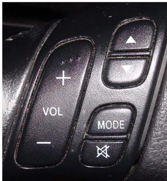
Steering wheel buttons. The “up” and “down” buttons send BUS+ messages to the tape deck (the ipod controller interprets them as track+ and track-).
