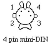
**Figure 2-1. TX/RX connector pin layout (4 pin mini-DIN male, wire side view)**
